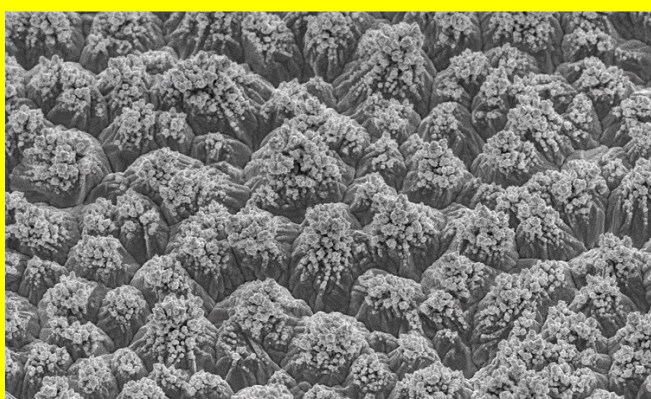
35µm treated-side Foil SEM × 1500
